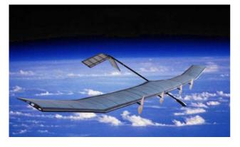
Figure 1. Scale model of the Pegasus platform
